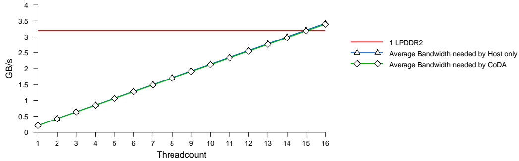
Fig. 8. Off-chip memory bandwidth usage We calculate the average off-chip memory bandwidth needed by all the benchmarks, and calculate how it scales when we run more and more threads, assuming a uniform random distribution among our benchmarks. Between the in-order, blocking nature of the L1 caches that limits the rate of misses, and the filtering effects of the L2 caches, the total off-chip bandwidth could be readily served by a small number of LPDDR2 channels.
